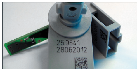
Left: Automotive switches. Material effect: color change. Laser marked with a fiber laser system.
