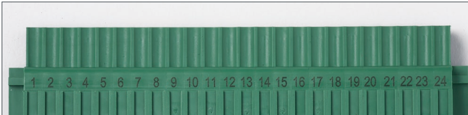
Terminal strip. Material effect: color change. This part was laser marked with a pulsed fiber laser marker.
